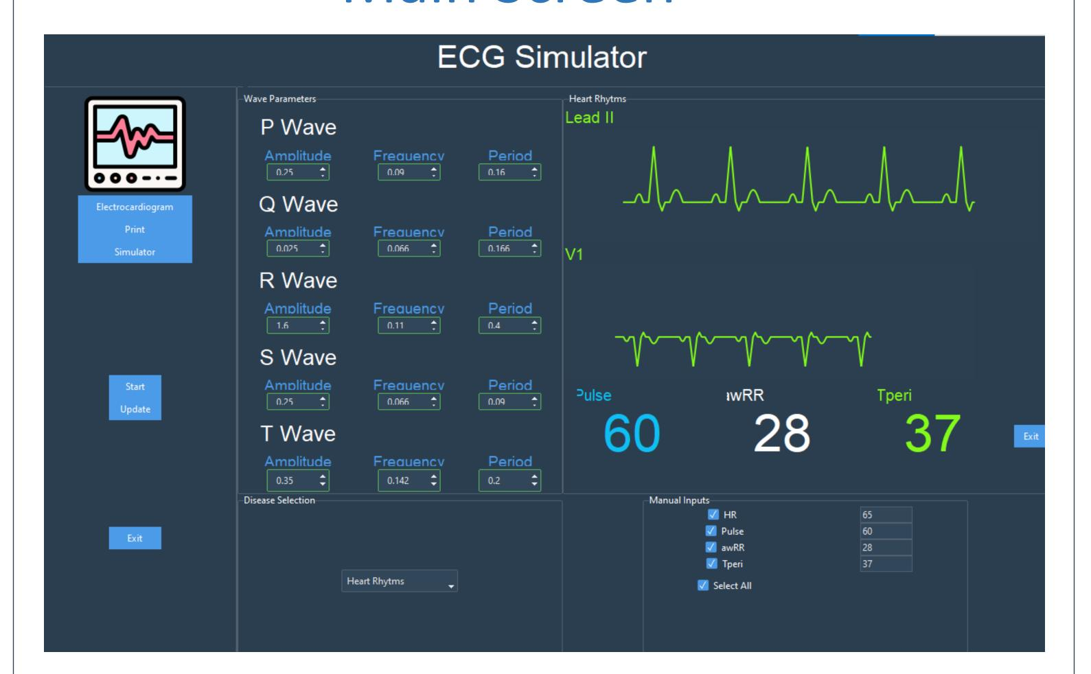
This is the screen used to generate the disease and adjust the parameters as needed. The GUI is used as a control center to create waves that can resemble a live patient who came in with heart problems.
