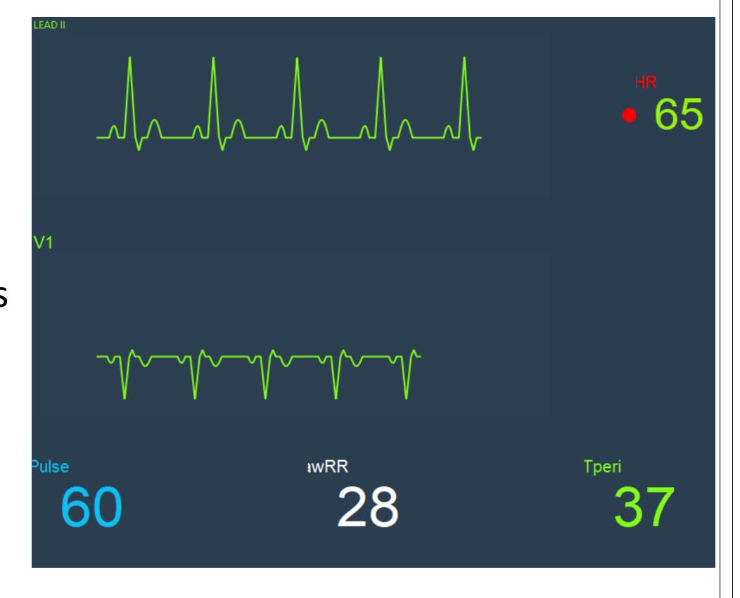
The ECG signal is animated based on the data points that were created by following the methodology from above. The updates are shown on the display once the wave returns to the left most part of the screen.
